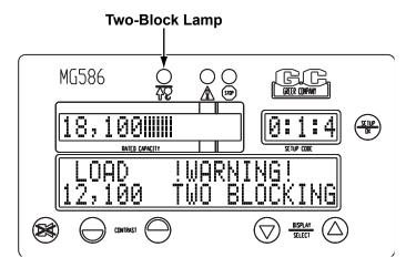
If the hook block is on a collision course with the head machinery at the end of the boom, the two-block lamp will illuminate and an audible alarm will sound continuously. The message: "!WARNING! TWO BLOCKING" will appear in the information window.
