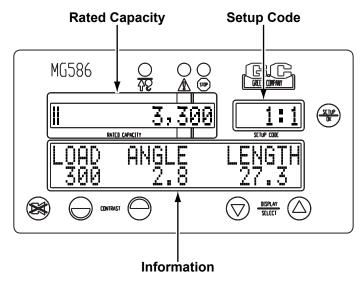
The current rated capacity for the crane in the current configuration will be displayed in the rated capacity window as well as the percent of rated capacity shown as a meter which progresses to the right as the load increases (see "Normal Operation" on page 7).
