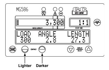
$Changes \ in \ temperature \ and \ lighting \ conditions \ may \ require \ adjustment \ of \ the \ display \ contrast.$
