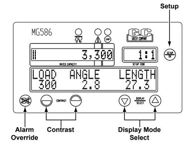
The **DISPLAY MODE/SELECT** keys are used to switch to different display formats showing various combinations of boom angle, boom length, and radius. They can also be used as an **UP ARROW** or **DOWN ARROW** key to scroll through menu selections.
