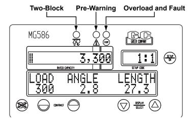
The red two-block lamp will illuminate when a two-block condition occurs (see "Two-Block Warning" on page 9).
