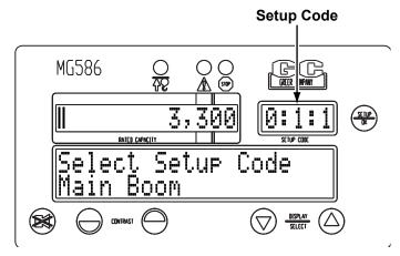
Following self-test, the system will go into the setup mode. The setup code window will display the same setup code used when the system was last powered off. Check that the correct setup code is displayed before operating the crane. Refer to "Configuration Selection" on page 6 for code setup instructions.
