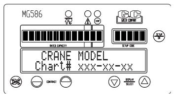
The information display will then show the crane model and capacity chart number for the system configured.
