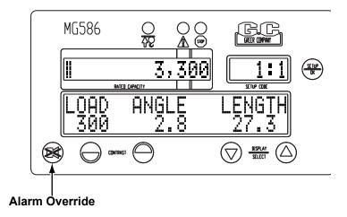
The alarm override button is used to temporarily disable current audible alarm conditions and to disable the automatic motion cutout. The audible alarm will sound again following any subsequent overload or two-block conditions, or any other alarm conditions.
