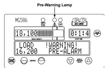
The system continuously monitors the weight of the load suspended below the boom head. The system compares this information with rated capacity data stored within the computer.
