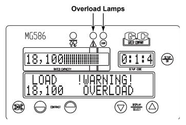
When the rated capacity of the crane reaches 100%, the percent of rated capacity meter moves from the caution (yellow-bordered) zone into the warning (red-bordered) zone.
