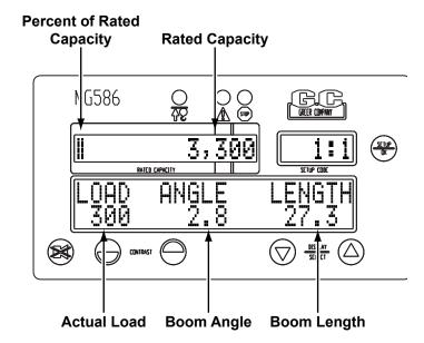
**Percent of rated capacity** indicates how near the operation is to full capacity and overload. The percent of rated capacity meter progresses to the right as the percentage increases. As long as the meter remains within the normal (green-bordered) zone, the percent of rated capacity is within normal operating limits. When the percent of rated capacity exceeds 60%, the rated capacity text will move to the left (see "Approaching Overload" on page 8).
