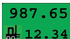
*The calculating of the partial load automatically begins when the 1<sup>st</sup> proximity is activated and will be completed when the 2<sup>nd</sup> proximity is then activated.*
