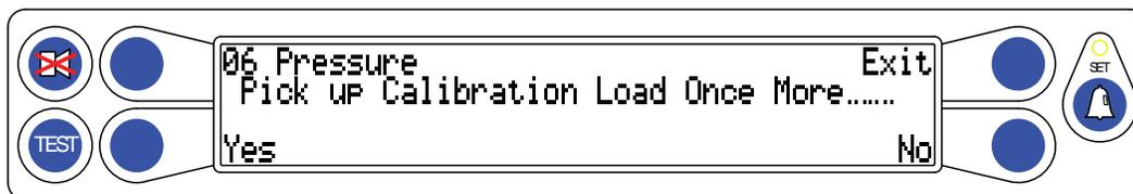
9. Press **Yes** to calculate the piston diameter and revert back to the main menu **06 Pressure**. This pressure routine is complete.
