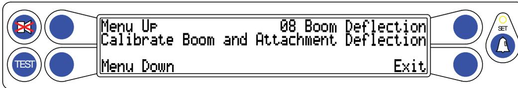
2. Press the **08 Boom Deflection** button to enter the routine and display the current “F” Factor in the center of the screen. The system will offer the opportunity to edit the existing “F” Factor or calibrate a new “F” Factor. It is not advisable to use the adjustment routine.
