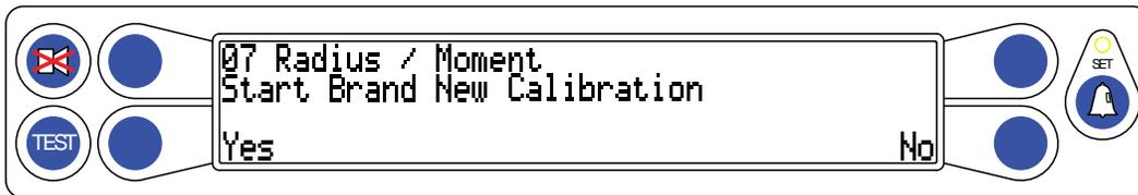
3. Press the **07 Radius/Moment** button will enter the Tare Load screen. Enter the weight of the downhaul. When entering the Tare load in the calibration routine, adding 100 pounds (0.1) to the actual weight will guarantee a slightly positive load reading in all operating configurations.
