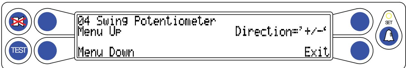
2. Press the “Direction = +/-” button to change the direction of the swing.
