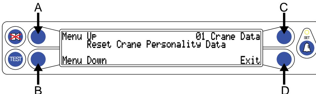
3. If there is no crane data present, or if the system has become corrupt, the display will read **“Personality not in use”**. In this case, proceed with the Crane data reset routine and reset the data.
