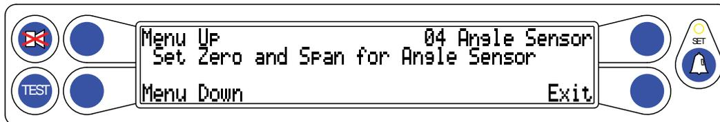
3. With the boom in a horizontal position, press the **Zero Angle? = XXX** button.
