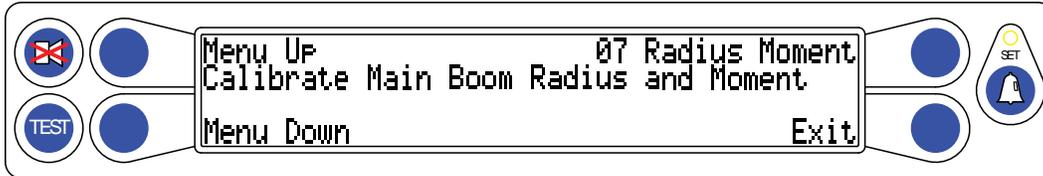
2. Press the **07 Radius Moment** button will give you a chance to enter an existing calibration in the edit mode, or start a brand new calibration. Press the **Yes** button to delete old calibration information and start a new calibration.
