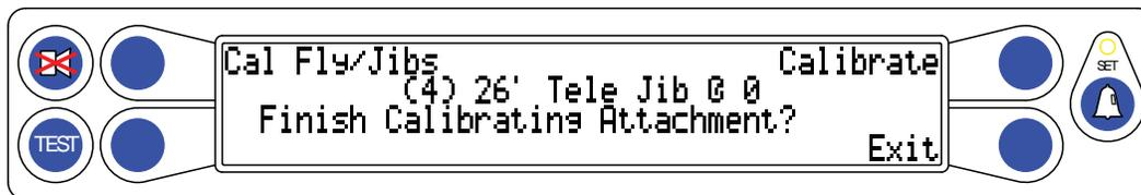
12. Press **Exit** to return to the normal operation mode. The system should display the proper radius and hook load. This is a sign that the jib calibration was successful.
