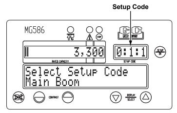
Following self-test, the system will go into the setup mode. The setup code window will display the same setup code used when the system was last powered off. Check that the correct setup code is displayed before operating the crane. Refer to "Configuration Selection" on page 7 for code setup instructions.
