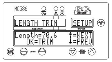
Press the **SETUP/OK** button to trim the length. The length measurement will be set to the exact length of the span and the extension number will be spanned in the computer calibration.
