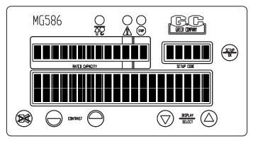
The information display will then show the crane model and capacity chart number for the system configured.
