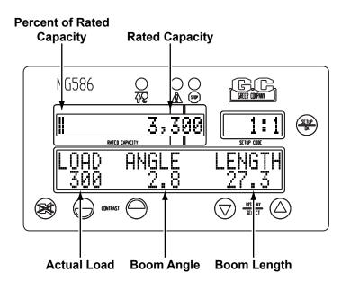
**Percent of rated capacity** indicates how near the operation is to full capacity and overload. The percent of rated capacity meter progresses to the right as the percentage increases. As long as the meter remains within the normal (green-bordered) zone, the percent of rated capacity is within normal operating limits. When the percent of rated capacity exceeds 60%, the rated capacity text will move to the left [see "Approaching Overload" on page 9].
