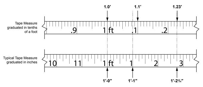
Note: The computer calculates measurements in feet and tenths of a foot, so having the correct measure will facilitate entering measurements.
