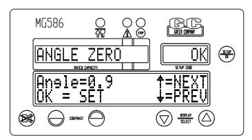
When the system enters calibration mode, the display will appear as in the illustration (angle reading may be different). Check to make sure the level on the boom is still at exactly zero degrees.
