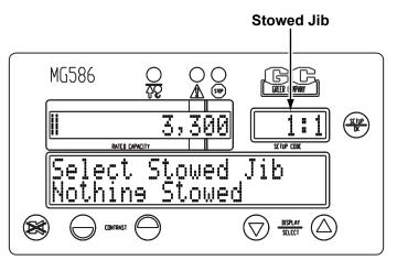
To select a different stowed jib, press the **UP ARROW** or **DOWN ARROW** key to display the desired option and press the **SETUP/OK** key to continue.
