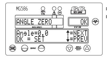
Press the **SETUP/OK** key to zero the system. Press the **UP ARROW** key to continue.
