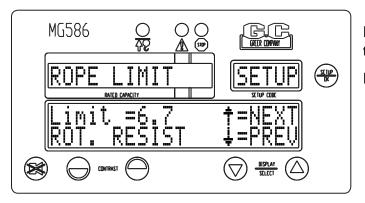
Press the **SETUP/OK** button to toggle between the types of cable.
