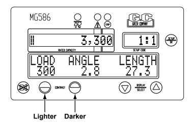
Changes in temperature and lighting conditions may require adjustment of the display contrast. Use the **CONTRAST** keys to lighten or darken the display as required.
