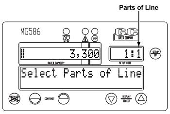
To change the parts-of-line, press the **UP ARROW** or **DOWN ARROW** key to select the desired number and press the **SETUP/OK** key to continue.
