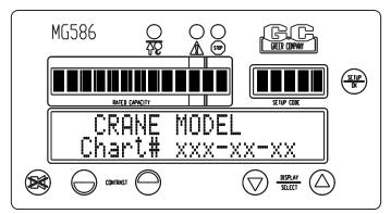
Following self-test, the system will go into the setup mode. The setup code window will display the same setup code used when the system was last powered off. Check that the correct setup code is displayed before operating the crane. Refer to "Configuration Selection" on page 7 for code setup instructions.
