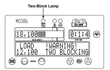
If the hook block is on a collision course with the head machinery at the end of the boom, the twoblock lamp will illuminate and an audible alarm will sound continuously. The message: "!WARNING! TWO BLOCKING" will appear in the information window.
