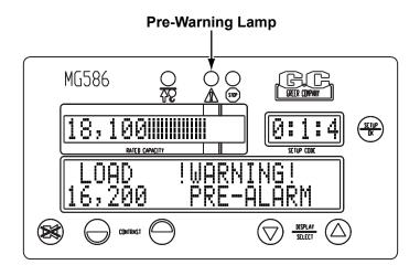
The system continuously monitors the weight of the load suspended below the boom head. The system compares this information with rated capacity data stored within the computer.
