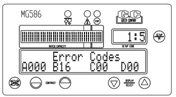
The codes will appear on the screen by group with a code number to define the specific fault. Refer to the repair manual for proper voltages and testing.
