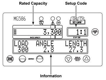
The current rated capacity for the crane in the current configuration will be displayed in the rated capacity window as well as the percent of rated capacity shown as a meter which progresses to the right as the load increases (see "Normal Operation" on page 8).
