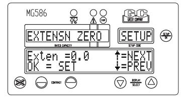
Press the **SETUP/OK** key to zero the span. Press the **UP ARROW** key to continue.
