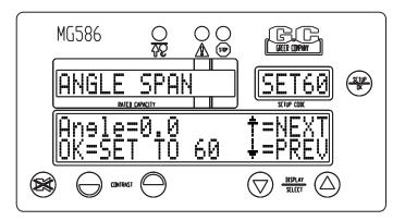
Press the **SETUP/OK** key to set the system to 60 degrees.
