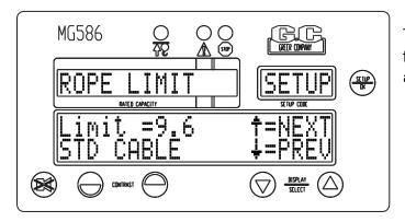
The system will display the proper cable limits for the type of cable selected. The cable types are preset from the crane configuration chart.
