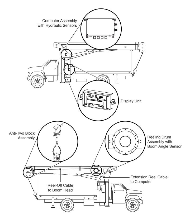
The **computer assembly** provides all of the functions necessary to read the system sensors, work out computations, and control the disconnect functions. In order to reliably calculate crane parameters, such as load and rated capacity, and interpret the crane capacity chart and code configuration numbers, information defining the physical characteristics of the crane has been loaded during factory setup.
