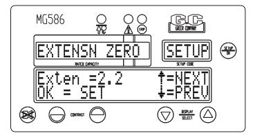
The display will appear as in the illustration (extension reading may be different). The extension sensor must be set to zero according to the procedure described previously.
