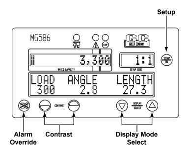
The **DISPLAY MODE/SELECT** keys are used to switch to different display formats showing various combinations of boom angle, boom length, and radius. They can also be used as an **UP ARROW** or **DOWN ARROW** key to scroll through menu selections.
